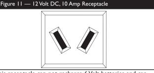
This receptacle can not recharge 6 Volt batteries and can not be used to crank an engine having a discharged battery. See the section "Charging a Battery" (page 11) before attempting to recharge a battery.
